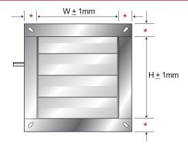
\* Where damper heights are requested in 100mm increments, the damper air way height will be 12mm greater for galvanised and stainless steel blades and 5mm greater for aluminium blades. Top and bottom flanges are amended to accommodate the blade profile, with the overall flange size being unaffected.
